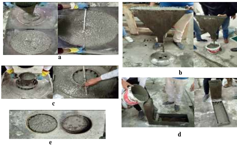
Fig., 2. The fresh properties of SCC mixes (a) The slump flow, slump flow time at T 50cm, (b) V-funnel test (Flow Time), (c) J-rang test tests (d) L-box test (Blocking Ratio) and (e) GTM screen stability.
